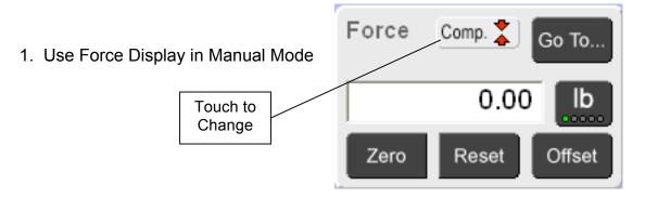
**NOTE:** This indicator is also present on **Quick Test** and **Automatic Mode** screens but does not allow convention change; its function is only as an indicator.
