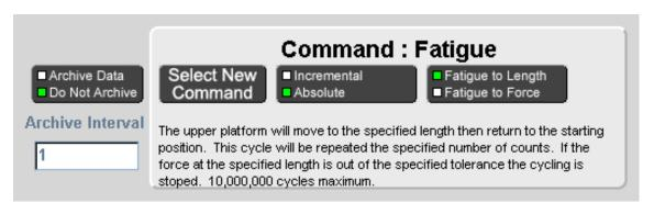
The fatigue test can be programmed to stop in the event of part fatigue or breakage. By entering a nominal force or length <u>and a tolerance value</u>, the part is checked when the platform stops at the target position. If the part does not test within the specified tolerance, the Fatigue test will stop.
