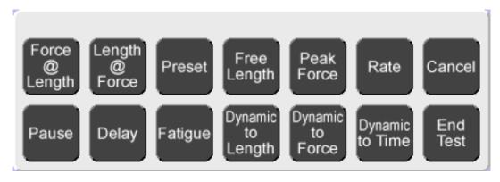
Choose test commands from this bar when creating a test sequence application. As a command is touched, a new gray box appears with the name of the command at the top. In each command box, select absolute or incremental testing and enter the required test point
