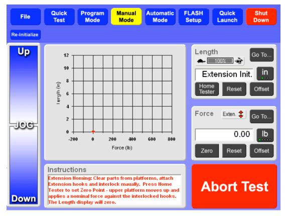
When setting the **Length Home Point** for extension, change the Compression setting to Extension. Touch the **[Comp.]** indicator in the **Force** display. (See section 4.2.2 about changing Compression and Extension testing.) The dialog box in the Length display will read **"Extension Init."** as shown above.
