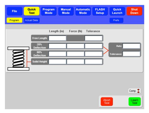
The **Program** screen allows you to run the generic **Quick Test** or manually enter data for the five test points and then run a test.
