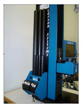
Optional thru-rod accessory kit mounted on machine (thru rod diameters ½" to 2")
