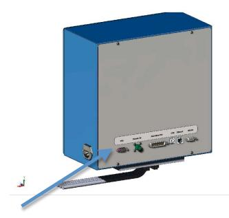
The FLASH head now includes an optional VGA connection to allow you to attach a video monitor to the tester and view operations from a remote location. A USB port allows connection to a monitor and keyboard for remote operation.
