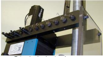
Extension hooks stored on machine for easy access (STAR 25)
