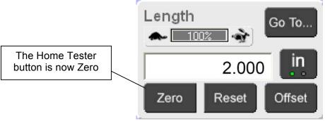
If the tester will only be used for compression testing, it is not necessary to set the length home point for extension. You are ready for compression testing.
