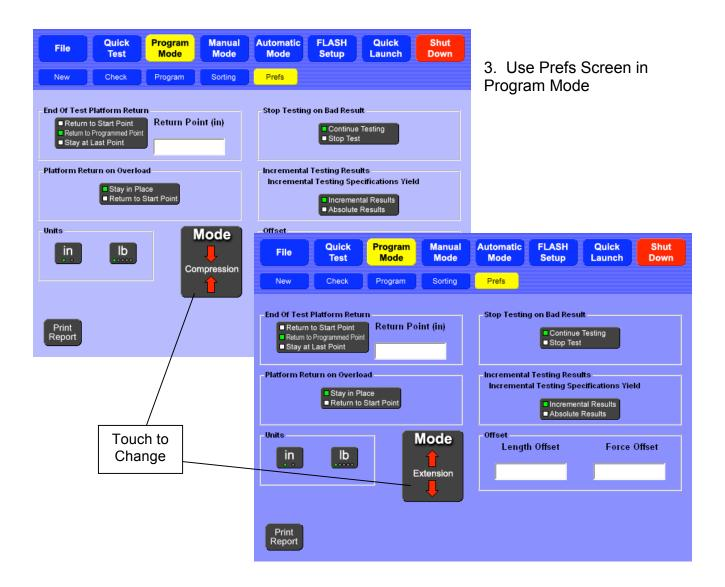
The tester will stay in the mode (convention) you select until you change it or the machine is turned off. You can navigate anywhere within the program and remain in the test mode selected, as indicated on each screen.
