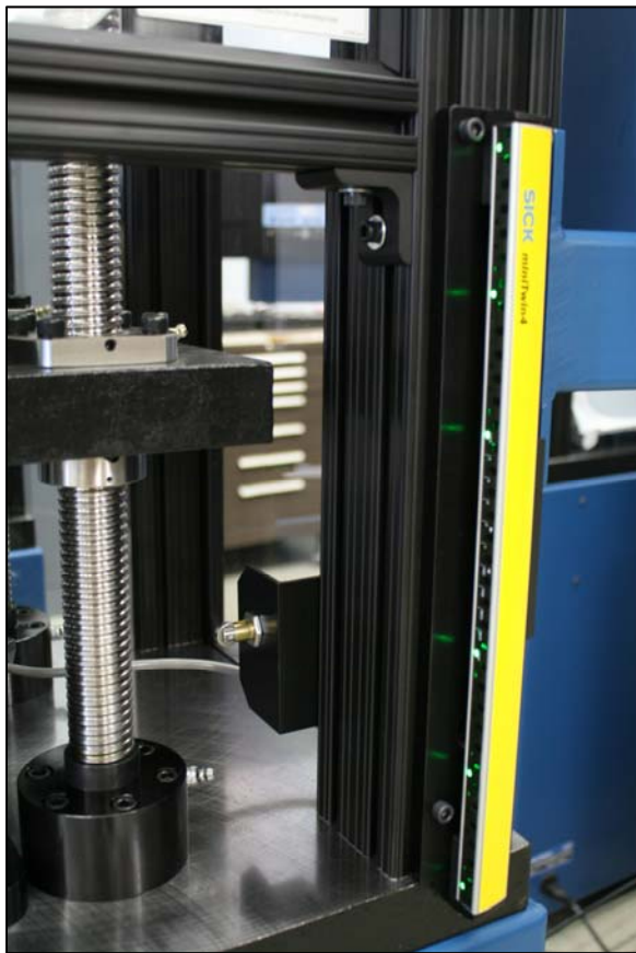
The above photos show the Light Curtain Guard active (left) and tripped (right).
